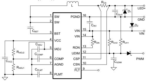
Figure 7-1. Typical Application Schematic
