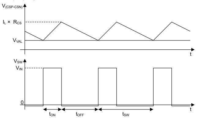
Figure 6-1. Adaptive On-Time Buck Converter Waveforms
