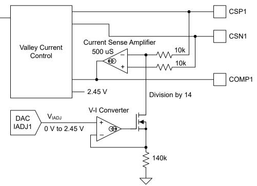
Figure 6-3. Closed-Loop LED Current Regulation
