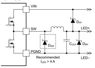
Figure 6-4. Switch node Schottky diode connection
