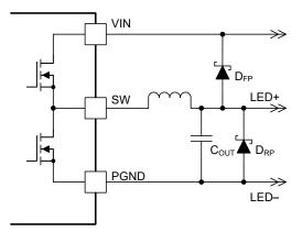
Figure 6-12. Transient Protection Using an External Diode
