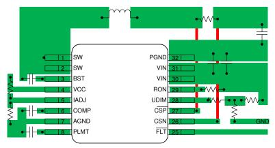
Figure 7-9. TPS92642-Q1 Layout Example
