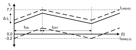
Figure 6-13. Overcurrent Protection Thresholds
