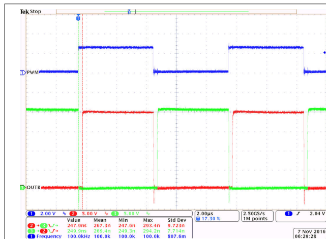
图 9-5. Bench Test Waveform for PWM and OUTA/B
