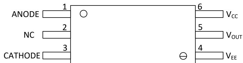
图 5-1. UCC23511 Package SO-6 Top View
