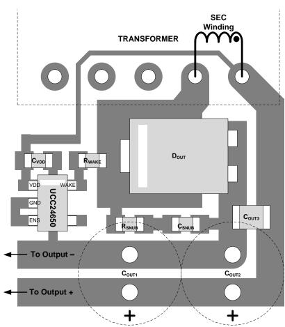
Figure 25. UCC24650 Partial Layout Example
