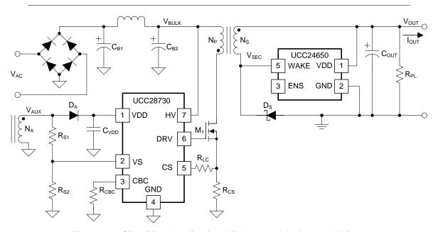
Figure 19. Simplified Application With Ground-Referenced Diode
