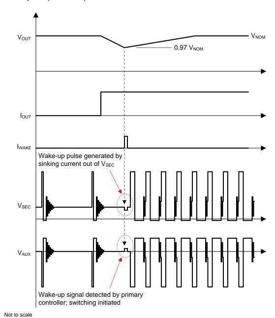
Figure 12. Simplified Timing Diagram of System Behavior
