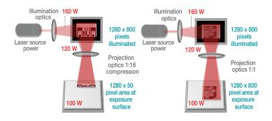
*Figure 9:* Optical compression as a means to attenuate power per pixel including a QR code (a) and a grayscale image (b).
