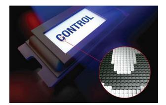
Figure 7: Individual mirror control for adaptive patterns.
