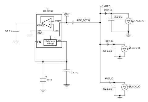
Figure 14. TINA-TI<sup>™</sup> Schematic for Voltage Reference Settling
