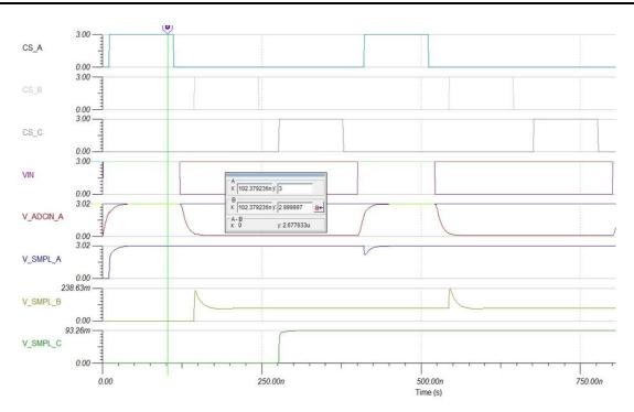
Figure 11. TINA-TI™ Simulation Results for Input Driver Settling
