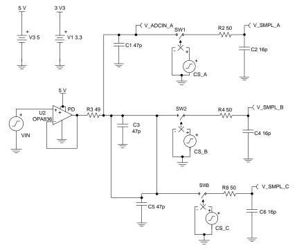
Figure 10. TINA-TI<sup>™</sup> Schematic for Input Driver Settling and Noise Analysis
