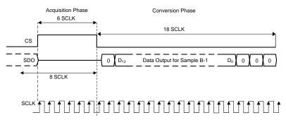
Figure 6. ADS7056 Timing Diagram for One Acquisition + Conversion Cycle
