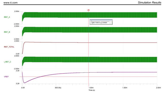
Figure 15. TINA-TI™ Simulation Results for Voltage Reference Settling
