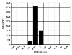
Figure 8. Gain Error Variation of ADS7056
