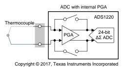
Figure 2. ADS1220 With Internal PGA
