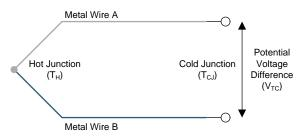
Figure 1. Basic Thermocouple Operation
