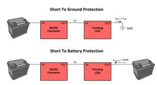
Figure 3. Two failure scenarios for off-board power supplies
