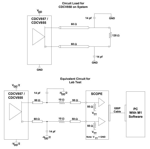
Figure 7. Testing Circuit
