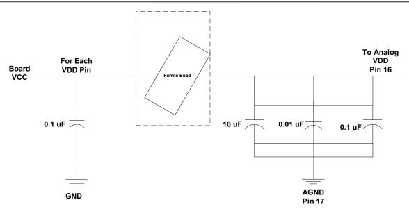
Figure 13. CDCV857/CDCV857A/CDCV855 Alternate Filter Circuit
