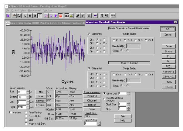
Figure 11. Selecting Channels to Measure Delay in M1
