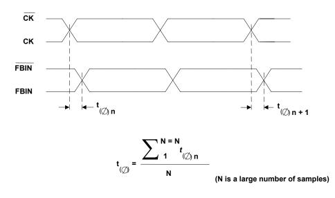
Figure 4. Static Phase Offset
