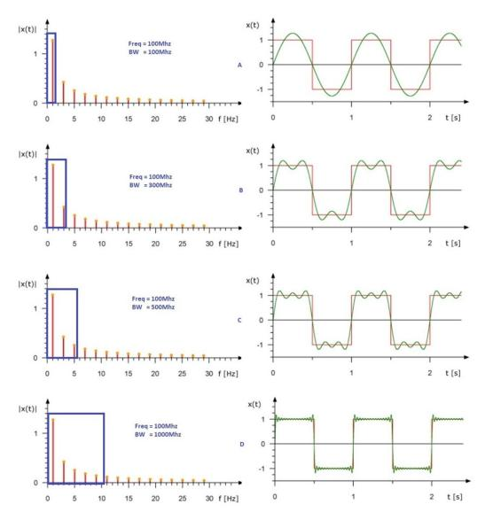
Figure 2. Square Wave with Different Harmonics
