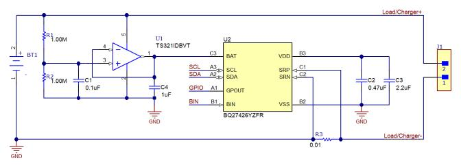
Figure 2-1. External Voltage Divider Using Operational Amplifier
