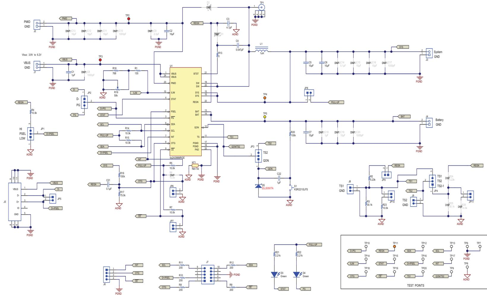
**Figure 11. bq24296M Schematic**
