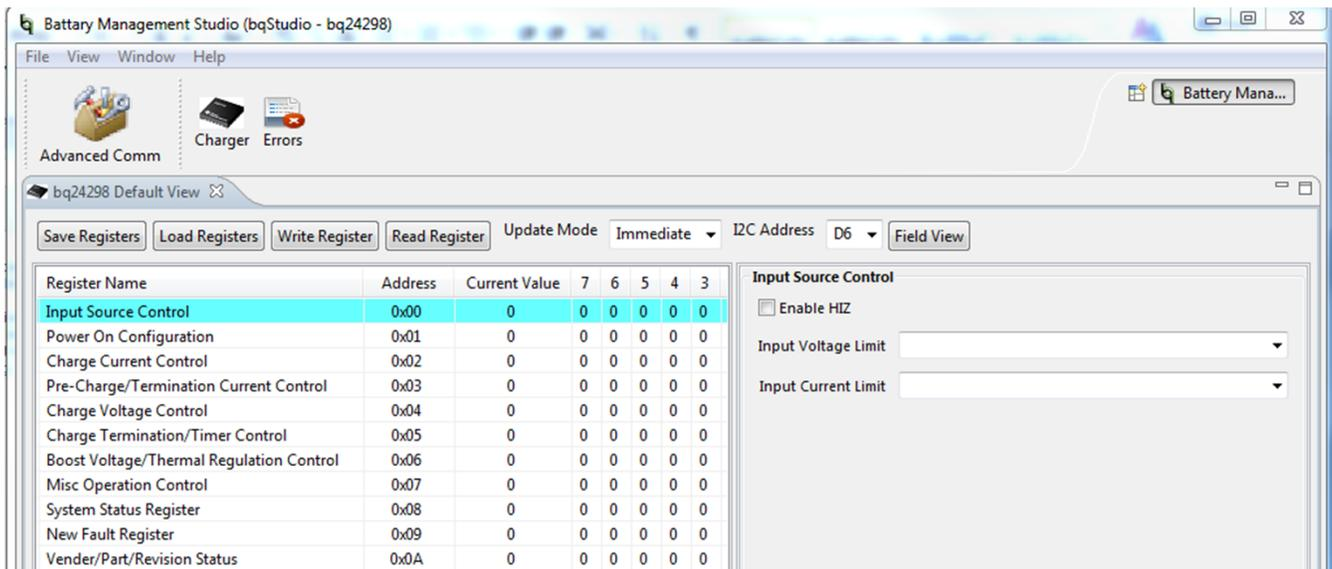
Figure 4. Main Window of the bq24298 Evaluation Software
