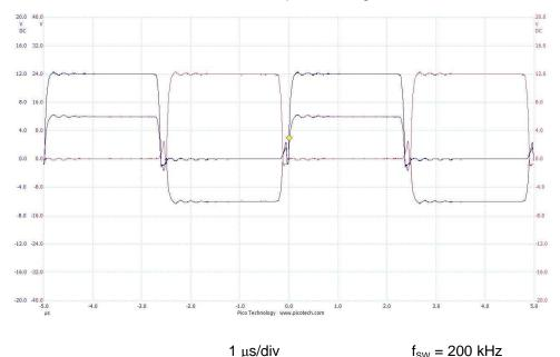
Figure 2. Primary-Side Phase Output Voltages (Red, Blue) of the Converter Phase-Phase Output is Computed (Purple) Showing the ±12-V Swing Across the Primary Side
