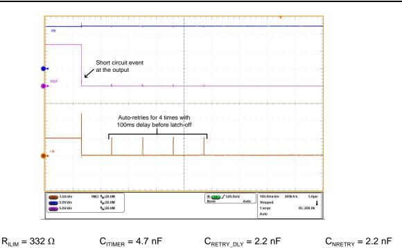
Figure 14. Output Hard Short-Circuit: TPS25982 Attempts Only Four Retries Before Latch-off
