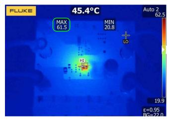
Figure 19. Case Temperature of the TPS25982 Device Under Sustained Fault with 1-sec Retry Delay
