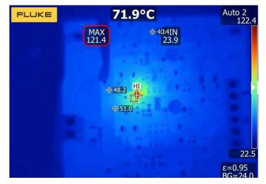
Figure 5. Case Temperature of the TPS259541 eFuse on the TPS2595EVM Under a Sustained Fault Condition
