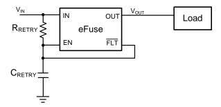
Figure 7. RC Network Delay at the EN Pin Sets the Retry Delay Time
