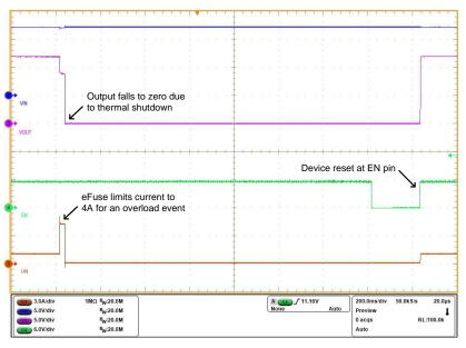
Figure 2. Latch-off Version of an eFuse (TPS259540) Waits for Power Cycle or EN Cycle
