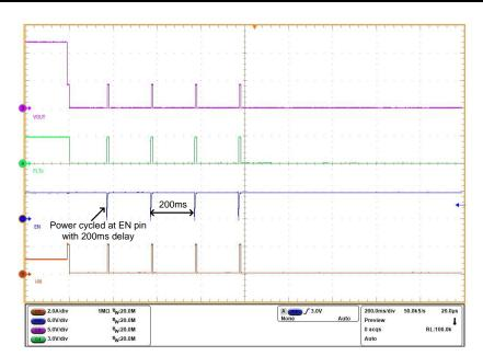
Figure 10. System Attempts Four Retries with 200-ms Retry Delay Before Latch-off
