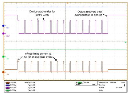
Figure 3. Auto-retry Version of an eFuse (TPS259541) Continues to Power the Cycle Until the Fault is Cleared
