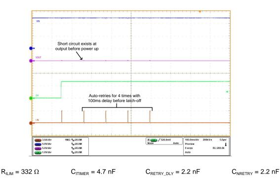
Figure 13. When Enabled into Short, the TPS25982 Attempts Only Four Retries Before Latch-off
