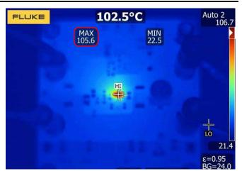
Figure 17. Case Temperature of the TPS25982 Device Under Sustained Fault with 100 ms Retry Delay
