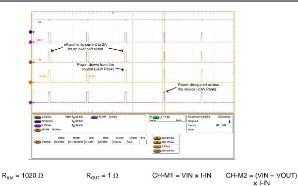
Figure 6. Power Dissipation Profile of the TPS259541 Under Sustained Overload Fault Condition
