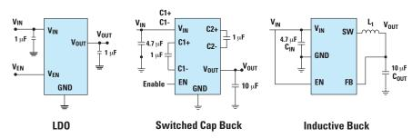
Figure 1: Common topologies for digital core power management
