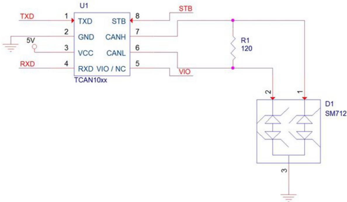
**Figure 4. TCAN10xx Transceiver with TVS Protection**
