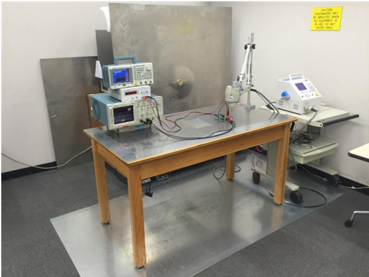
Figure 3. IEC ESD-compliant Test Setup
