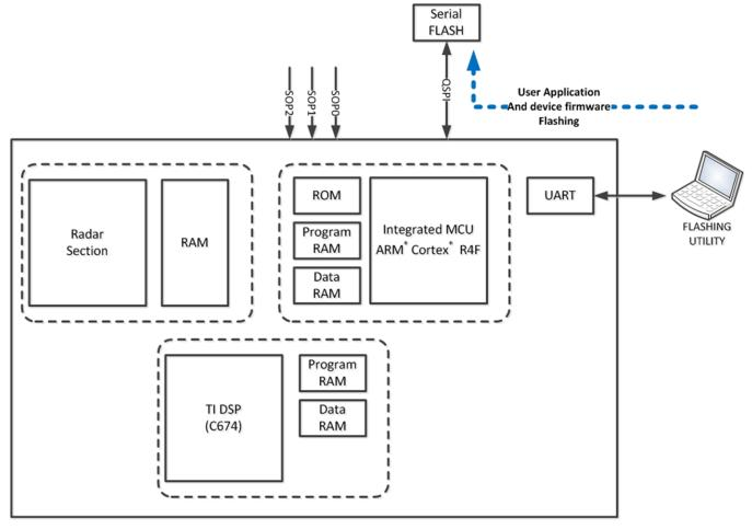
Figure 2. Flashing Mode of Bootloader
