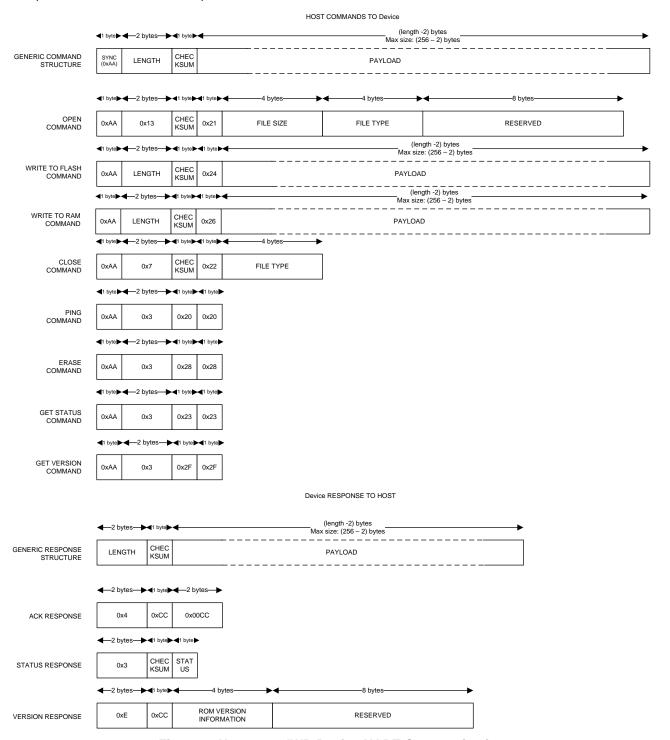
Figure 8. Host  $\leftarrow \rightarrow$  IWR Device UART Communication
