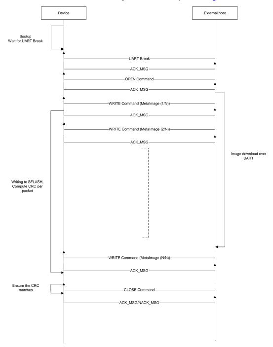
Figure 9. Flashing Sequence
