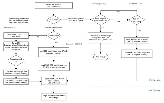
Figure 4. Basic Bootloader Flow Chart
