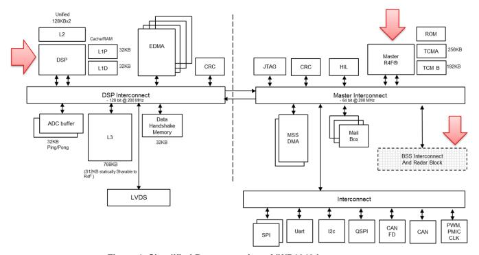
Figure 1. Simplified Representation of IWR1642 Interconnect
