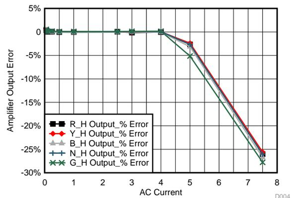
图 33. Current Versus Output Error for High Gain Amplifier Using OPA4314
