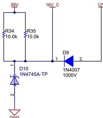
图 11. Comparator Power Supply Generated From 39-V Supply
