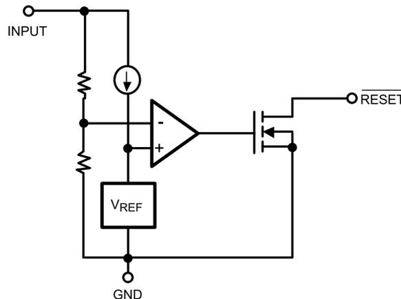
图 7. LM8364 Functional Block Diagram
