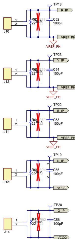
图 15. Current Input Connector With Burden Resistor
