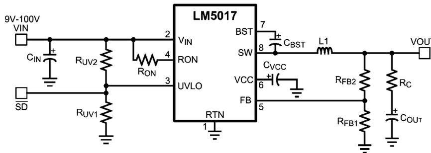
图 8. LM5017 Typical Application Diagram
