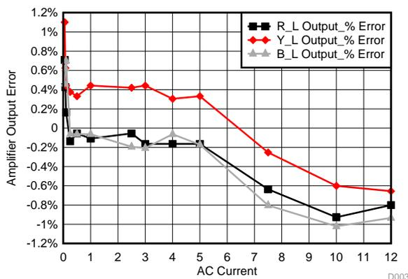
图 32. Current Versus Output Error for Low Gain Amplifier Using OPA4314
