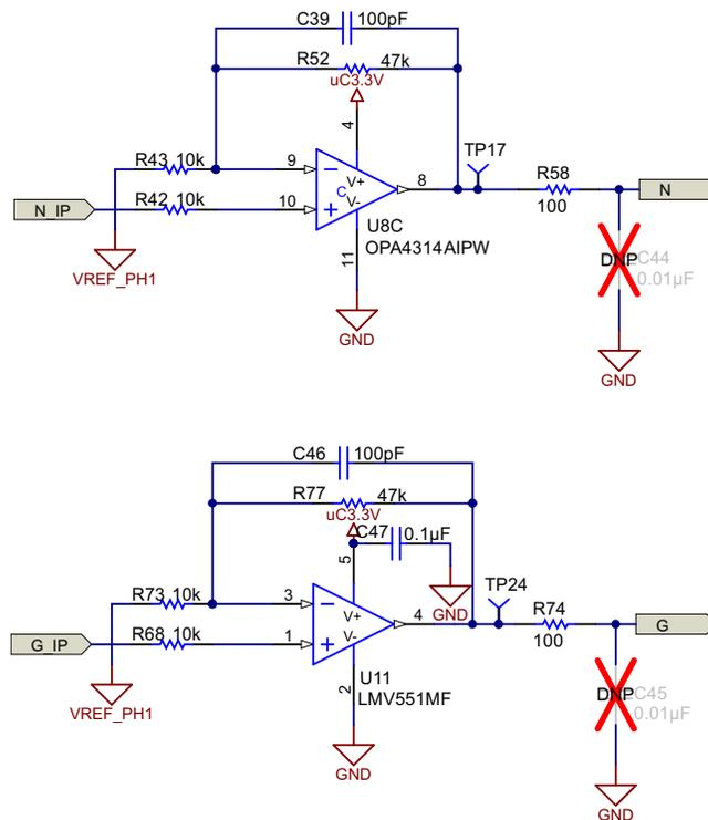
图 17. Amplifier With Single Gain Schematic
