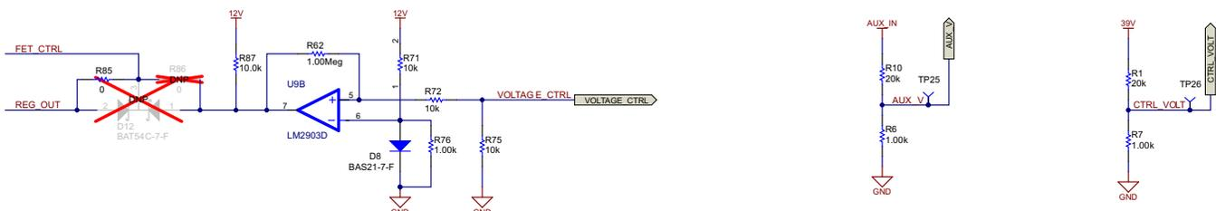
图 13. Comparator for PWM Control and DC Supply Voltage Sensing Schematic
