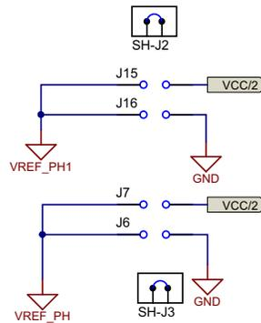
图 19. Jumper for AC Current or Rectified Current Schematic
