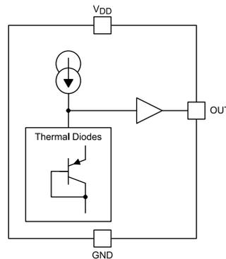
图 6. LMT87 Functional Block Diagram
