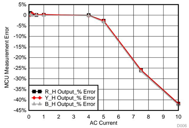
图 35. High Gain Measurement Error With Internal 12-Bit ADC
