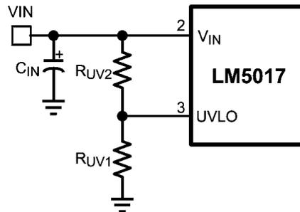
图 12. UVLO Resistor Setting
