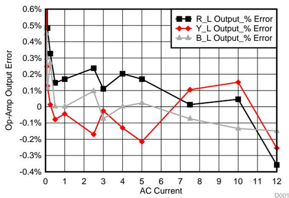
图 30. Current Versus Output Error for Low Gain Amplifier Using LMV614
