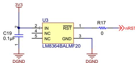
图 22. Undervoltage Sense Input to MCU Schematic
