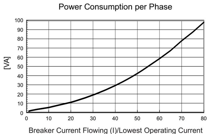
**图 1. Typical Power Consumption for Current and Lowest Operating Current**
