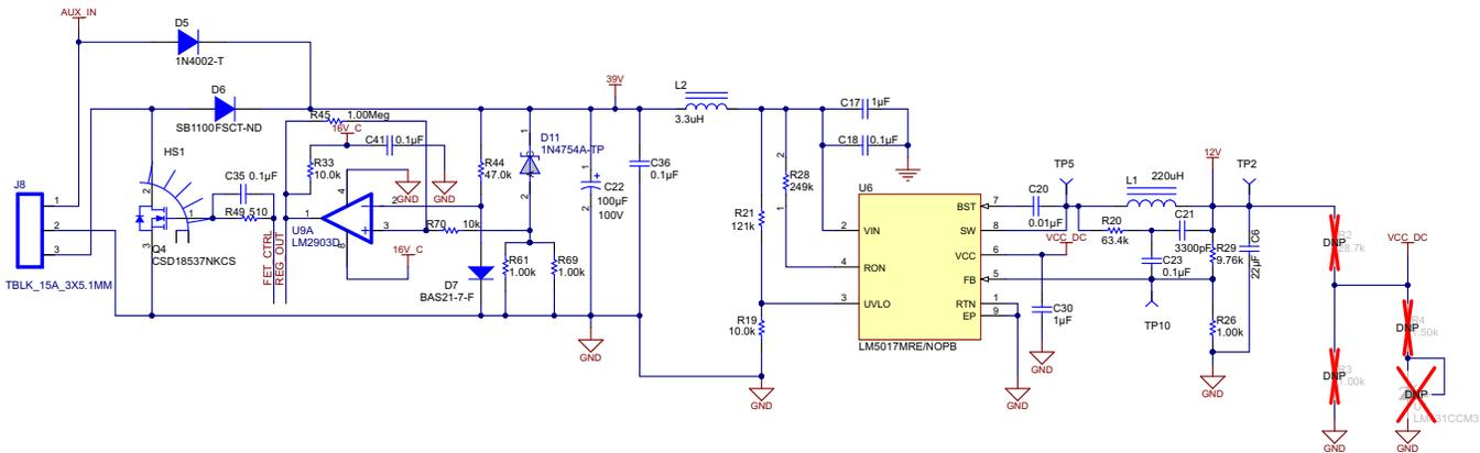
图 10. Self-Power Supply Including DC-DC Converter Schematic
