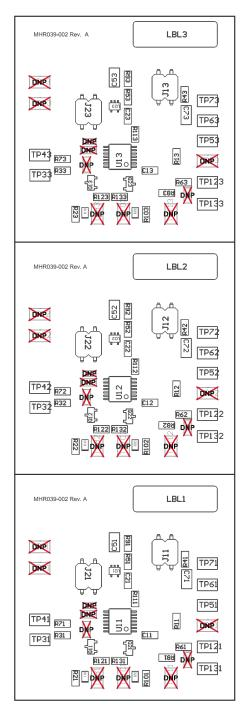
Figure 3. PCB Component Placement
