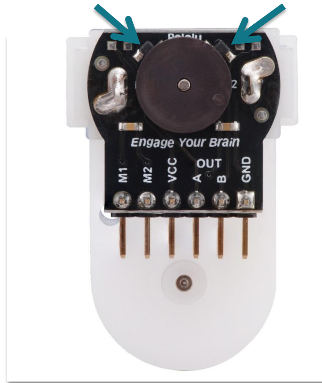
Gearmotor and Encoder Assembly for Romi/TI-RSLK MAX robot kit
