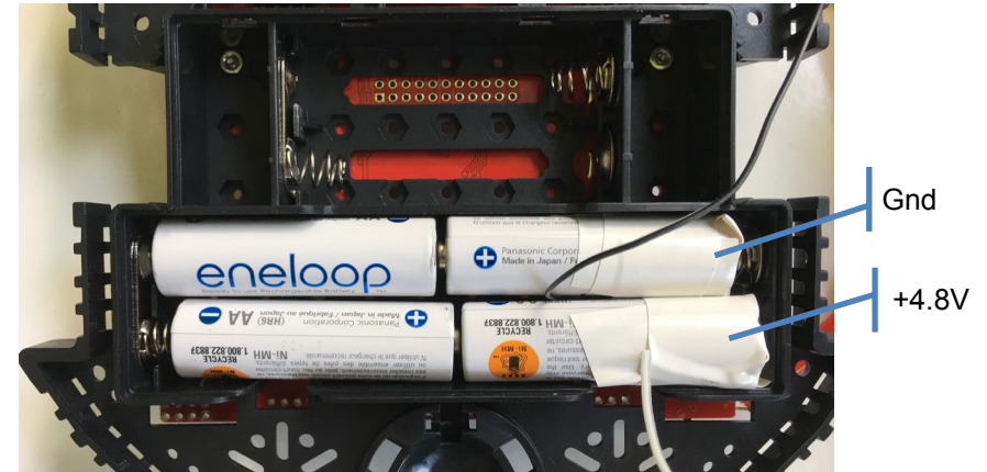
Figure 3. TI-RSLK chassis holding 4 AA batteries.
