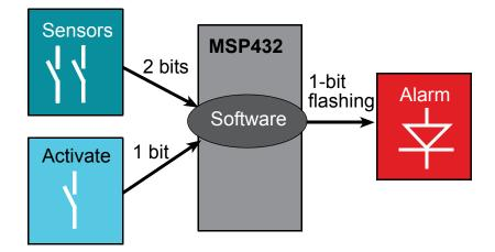
Figure 8.1. Window Intruder Detector Alarm System.
