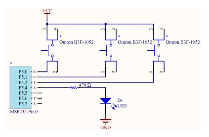
Figure 8.6. Hardware schematic interfacing input and output pins.
