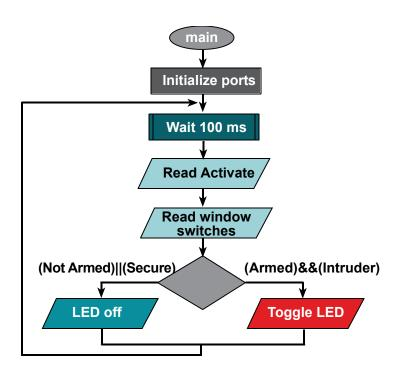
Figure 8.7. Possible software algorithm for the system drawn as a flowchart.
