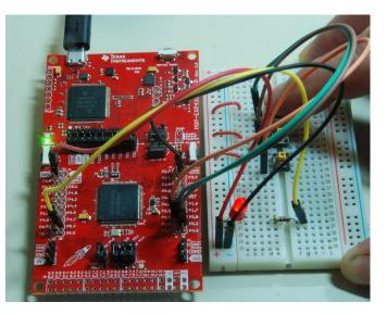
Figure 8.2.MSP432 LaunchPad (non-modified) and external circuits
