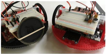
Figure 1. Sound output on one robot and sound input on the other.
