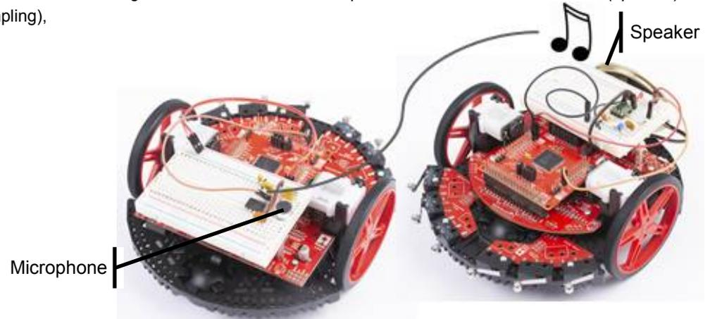
Figure 1B. Sound out of one robot and into the other (option B).
