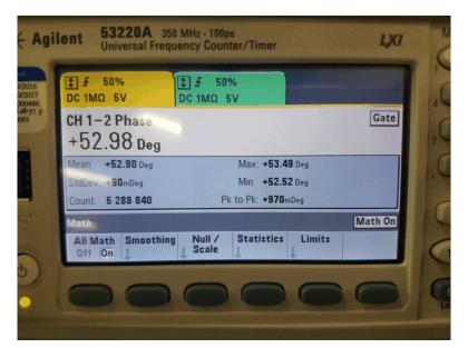
Figure 4. Phase at Room Temperature
