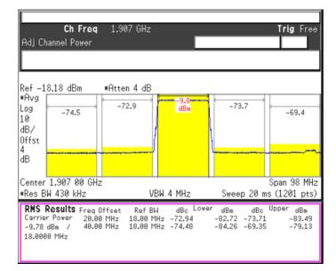
Figure 8. Clean ACPR Measurement Directly From DAC38RF82
