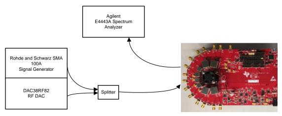
Figure 10. Hardware Setup for Jammer Simulation
