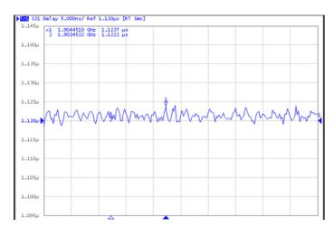
Figure 5. Latency Measurement, Average Latency = 1.12 µs
