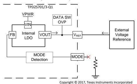
Figure 3. MODE Pin Fault
