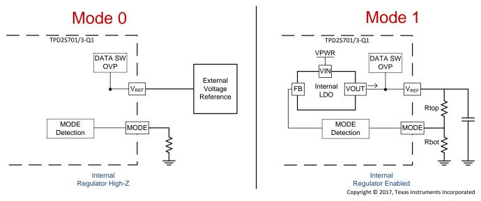
Figure 2. Mode Functionality Block Diagram
