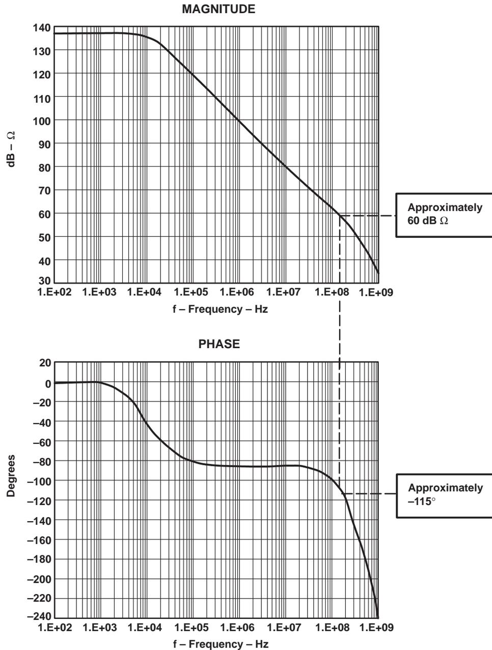
**Figure 3. THS3001 Open Loop Transimpedance**
