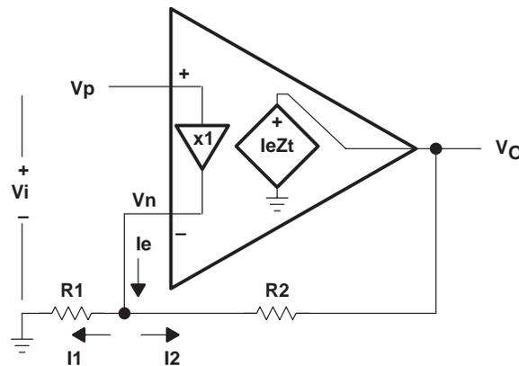
**Figure 1. Noninverting Amplifier Using Current Feedback Model**
