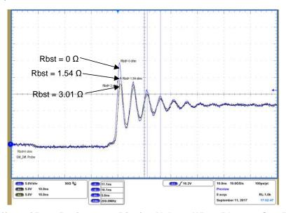
Figure 10. Affect of Boot Resistors on Ringing Voltage When Rbst = 0  $\Omega$ , 1.54  $\Omega$ , and 3  $\Omega$
