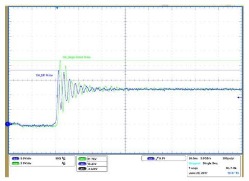
Figure 3. Typical Switch Ringing Waveform of TPS53319 Device
