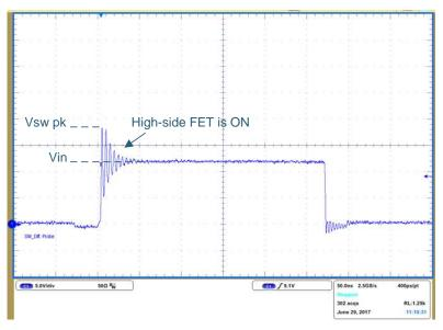
Figure 6. Switch Ringing Waveform Rising and Falling Edges
