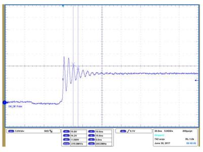
Figure 7. Switch Node Ringing Waveform Without Snubber
