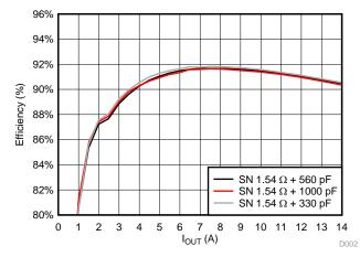
Figure 12. Efficiency Comparison When Snubber Capacitance-Cs Changes
