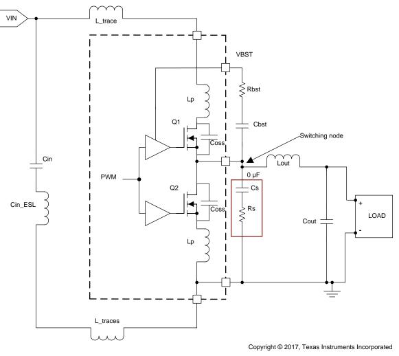
Figure 4. RC Snubber Added Circuit With Parasitic Components
