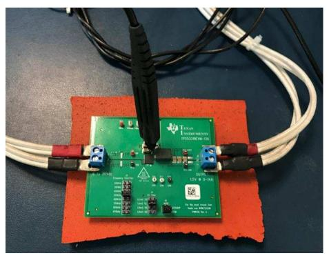
Figure 2. 1-GHz Differential Probing
