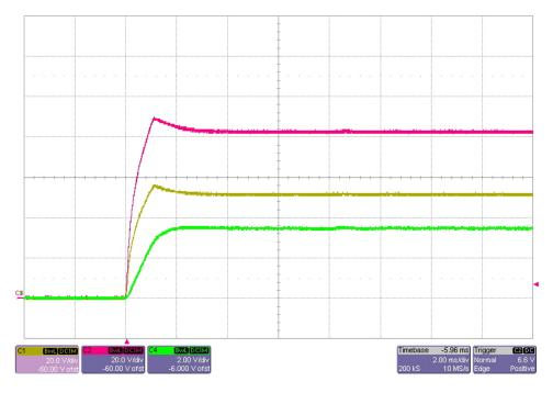
The 82V, 52V and 3.7V output voltage startup waveforms are shown in the figure below after the application of 14Vin. The outputs voltages were loaded to max. The 3.7V output was measured with respect to the GND (3.7V output voltage is offset by 8.2V zener diode D6). (82V/52V = 20V/DIV, 3.7V = 2V/DIV, 10mS/DIV)
