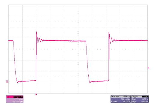
The photo below shows the switch node voltage (TP6) of the 82V converter. The dithering circuit is operational. The outputs were loaded to max loads. Vin = 14V. (5V/DIV, 2uS/DIV)
