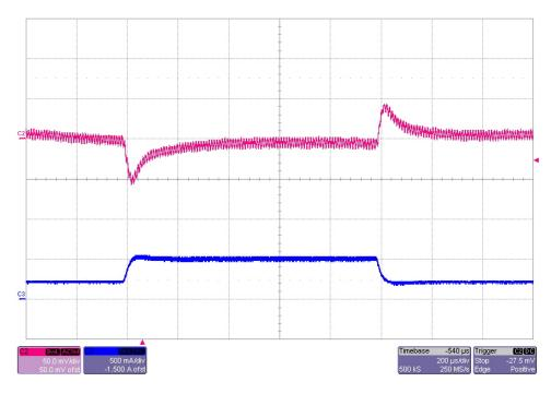
The photo below shows the 82Voutput response and recovery to a 30mA to 40mA step load. Vin = 14V. (1V/DIV, 20mA/DIV, 500uS/DIV)
