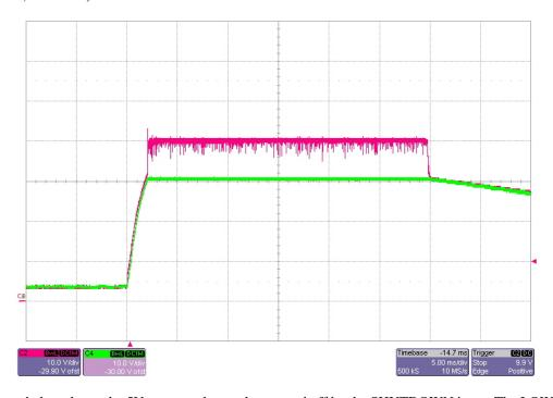
The photo below shows the 5V output voltage when turned off by the SHUTDOWN input. The LOWBAT transitions low below its set point of 3.3V. The 5V output was loaded to 0.2A and Vin = 14V. (5V = 1V/DIV, LOWBAT = 2V/DIV, 1mS/DIV)
