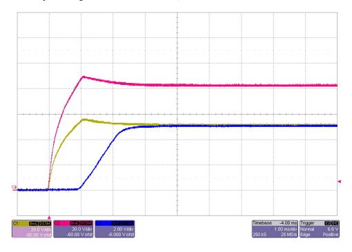
The 82V, 52V and 5V output voltage startup waveforms are shown in the figure below after the removal of the Shutdown signal. Vin = 14Vin. The 82V and 52V outputs voltages were loaded to max and the 5V was loaded to 1mA. The linear regulator is holding up the output voltage at 4.5V before the 5V output turns on. (Shutdown = 5V/DIV, 82V/52V = 20V/DIV, 5V = 2V/DIV, 1mS/DIV)
