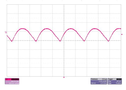
The 52V output ripple voltage is shown in the figure below. The image was taken with all outputs loaded to max load (5V @ 0.5A, 82V @ 30mA, 52V @ 40mA, 3.7V @ 0.5A). Vin = 14V (500mV/DIV, 5uS/DIV)
