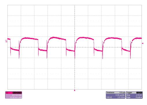
The 82V output dither frequency ripple voltage is shown in the figure below. The image was taken with all outputs loaded to max load (5V @ 0.5A, 82V @ 30mA, 52V @ 40mA, 3.7V @ 0.5A). Vin = 14V (500mV/DIV, 500uS/DIV)
