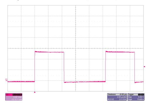
The photo below shows the switch node voltage (TP11) of the 5V converter. The dithering circuit is operational. The outputs were loaded to max loads. Vin = 14V. (5V/DIV, 2uS/DIV)
