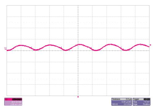
The 5V output dither frequency ripple voltage is shown in the figure below. The image was taken with all outputs loaded to max load (5V @ 0.5A, 82V @ 30mA, 52V @ 40mA, 3.7V @ 0.5A). Vin = 14V (20mV/DIV, 500uS/DIV)
