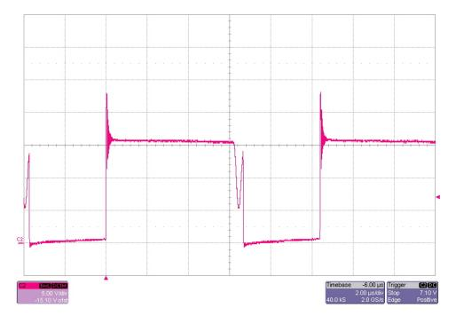
The photo below is of FET Q1 switch node (TP11). The input voltage is 14V and the outputs are loaded at 0A. (5V/DIV, 2uS/DIV)
