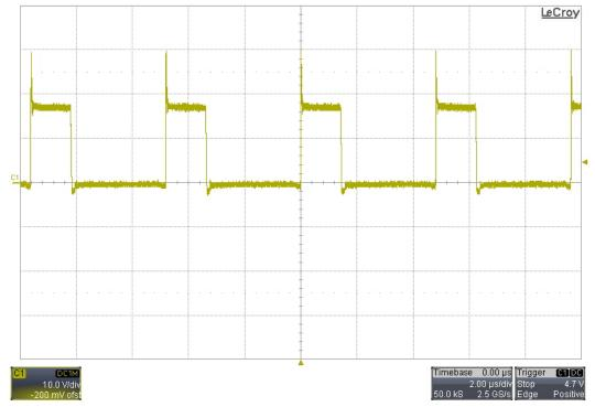
10.2 Q3 Synchronous FET Vds – 250VDC Input, 20A Load
