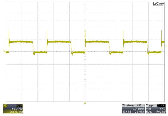
10.4 Q10 Synchronous FET Vds – 250VDC Input, 20A Load
