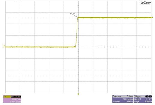
The scope plot below shows the 5V output voltage startup waveform after the application of 48Vdc at J2 (PoE). The output was loaded to 5.0A.
