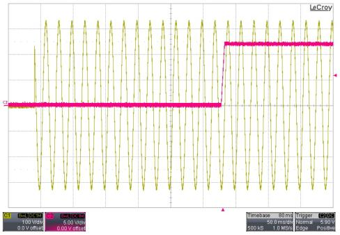
6.2 230VAC/50Hz Startup – 48Ω Load
