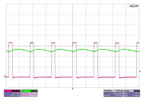
The photo below shows the (Q1) FET switch node and the LED current. The image was taken with an output of 8 LEDs and regulated to 0.515A. The input voltage was set to 12V. (10V/DIV, 200mA/DIV, 2uS/DIV)
