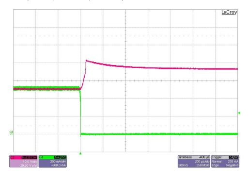
The photo below shows the LED Anode voltage (with respect to ground) and the LED current during an open LED test. The image was taken with an output of 8 LEDs and regulated to 0.515A. The input voltage was set to 36V. (10V/DIV, 200mA/DIV, 200uS/DIV)
