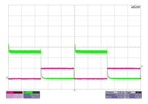
The photo below shows an external PWM input (50%) and the LED current. The image was taken with an output of 8 LEDss and regulated to 0.515A. The input voltage was set to 36V. (5V/DIV, 200mA/DIV, 1mS/DIV)
