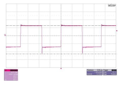
The photo below shows the 12V main secondary Rectifier (D1) switching voltage with the diode snubber **removed** (for reference). The input voltage is 57V and the output is loaded to 5A. (10V/DIV, 1uS/DIV)
