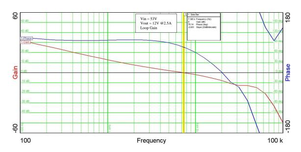
The plot below shows the 12V loop gain and phase margin with the output loaded to 2.5A (without load share controller and C22 = 2200 pF, R132 = 0). The input voltage was set to 53V.
