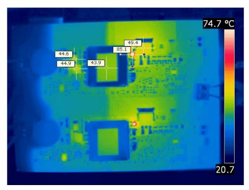
A thermal image is shown below when operating in parallel at 53V input and 10A output (5A each flyback), with no airflow.
