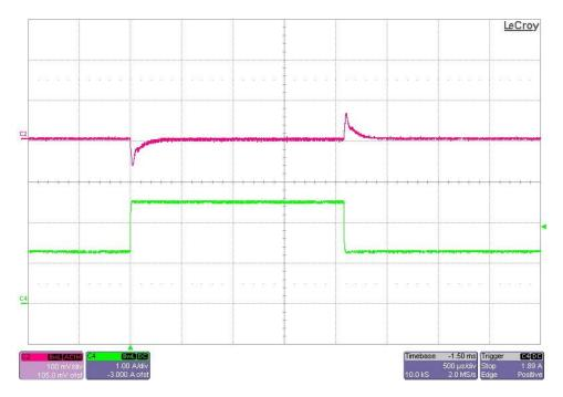
The photo below shows the single flyback output voltage (ac coupled) when the load current is stepped between 2.5A and 5A. Vin = 53V. (100mV/DIV, 2A/DIV, 500uS/DIV)
