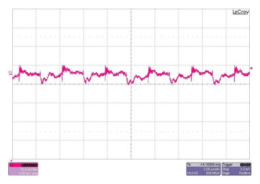
The 12V output ripple voltage is shown in the figure below. The image was taken with the output loaded to 5A. The input voltage is set to 53V. (10mV/DIV, 2uS/DIV)
