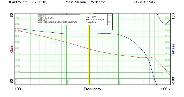
The plot below shows the 12V loop gain and phase margin with the output loaded to 5A (without load share controller and C22 = 2200pF, R132 = 0) and 800uF additional output cap added. The input voltage was set to 53V.
