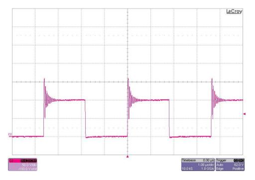
The photo below shows the 12V primary FET switching voltage. The input voltage is 57V and the output is loaded to 5A. (50V/DIV, 1uS/DIV)
