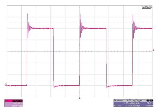
The photo below shows the 12V primary FET switching voltage. The input voltage is 57V and the output is loaded to 2.5A. (20V/DIV, 1uS/DIV)
