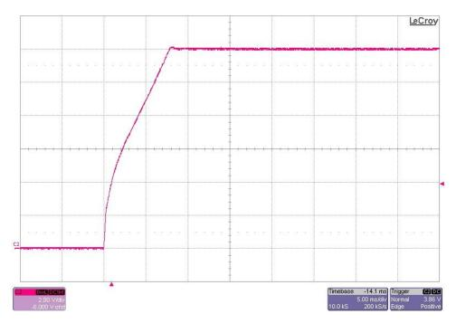
The photo below shows the output voltage startup waveform of a single flyback after the application of 53V in. The 12Voutput wase loaded to 2.5A. (2V/DIV, 5mS/DIV)
