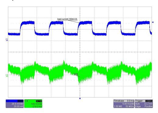
Input voltage = 375VDC Output load = 0.2 to 0.4A
