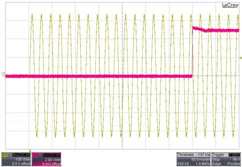
6.3 115VAC/60Hz Startup – 2.5Ω Load
