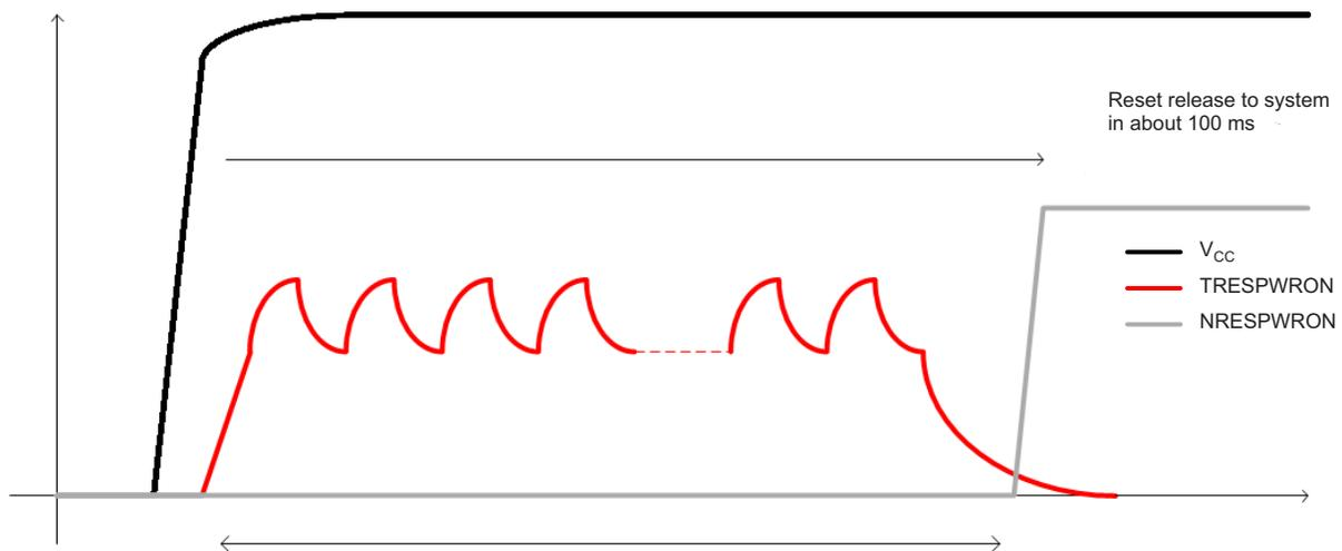
Note: The TRESPWRON signal has around 100 charges and discharges to monitor the reset signal releasing in accord with the TPS65023-Q1 specifications.
