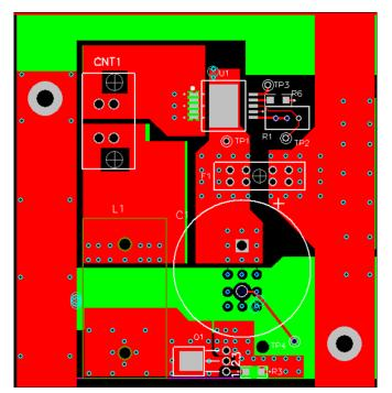
Figure 7. Layout of Driver Board
