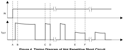
Figure 4. Timing Diagram of Hot Repetitive Short Circuit
