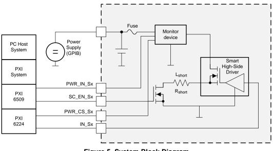
Figure 5. System Block Diagram
