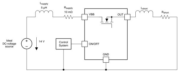
Figure 1. Smart HSS Short-Circuit Model
