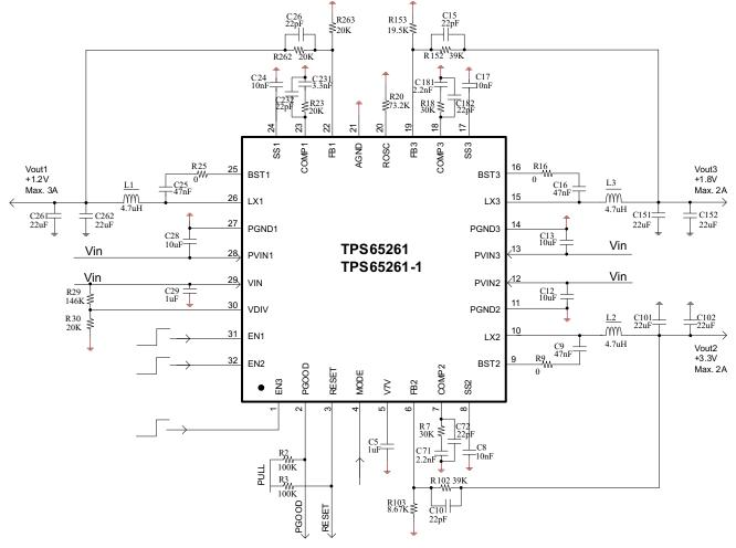
Figure 5. TPS65261 Typical Application Circuit
