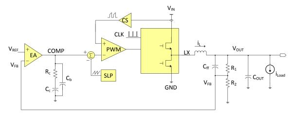
Figure 1. PCM BUCK Converter Block Diagram
