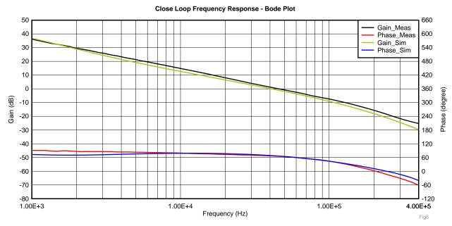
Figure 6. Measured Bode Plot vs. Calculated Bode Plot
