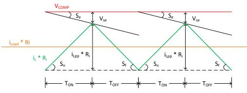
Figure 3. PWM Comparator Input Signals
