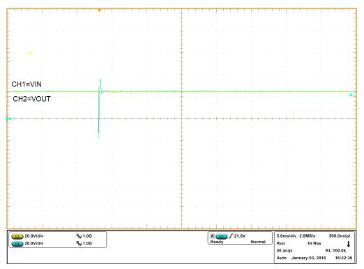
Figure 10. Protection from Negative Surge [–500 V,  $Z_i$  = 42  $\Omega$ ]
