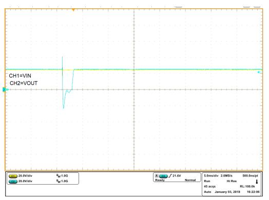
Figure 9. Protection from Positive Surge [500 V,  $Z_i$  = 42  $\Omega$ ]
