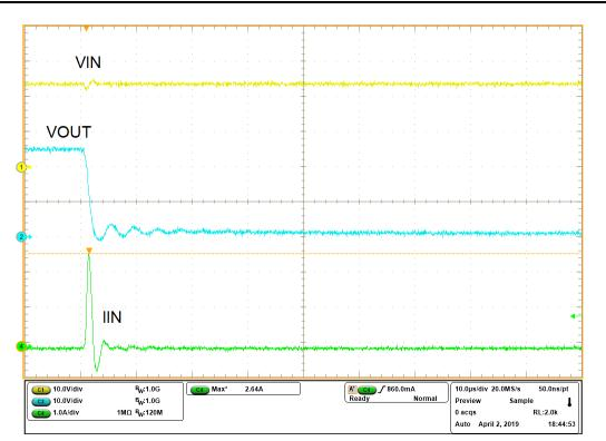
Figure 7. Short Circuit Protection with TPS2662 Devices
