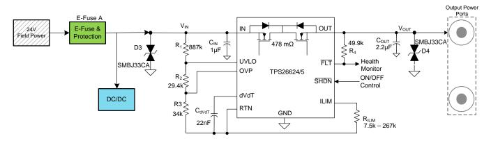
Figure 5. Output Power Port Protection with TPS2662
