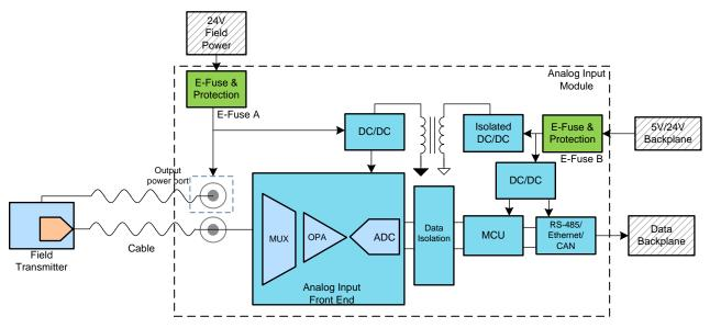
Figure 1. Analog Input Module with Output Power Port
