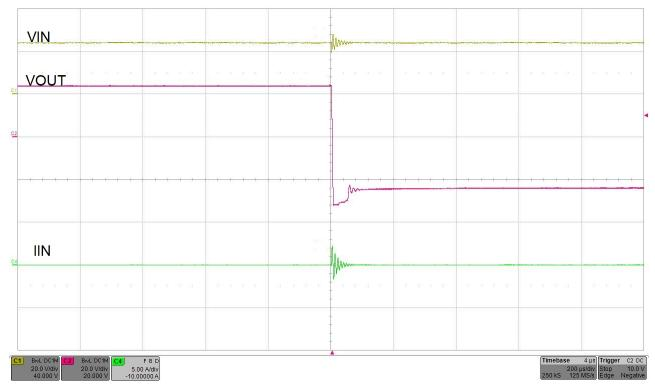
Figure 6. Output Reverse Polarity Protection with TPS26624 and TPS26625
