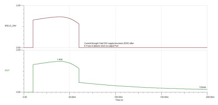
Figure 4. Response on Reverse Polarity
