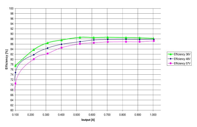
Efficiency Curve for Vin = 36 V, 48V, 57V
