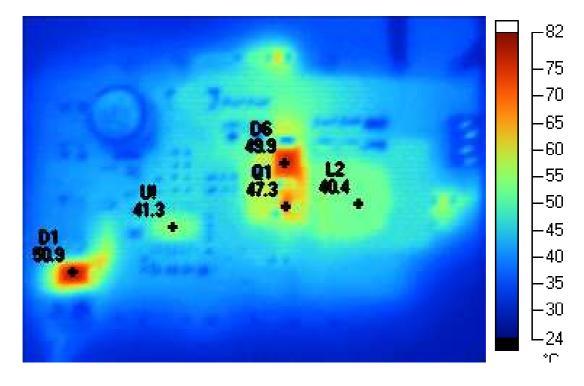
Fig.8 Thermal picture with hot spots at Vin=36V@lout=1A
