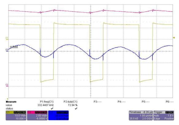
Fig.4 C1: Vds\_Q1, C2: V\_in ripple (scope probe on Aux\_Power J1+), C3: Vout ripple
