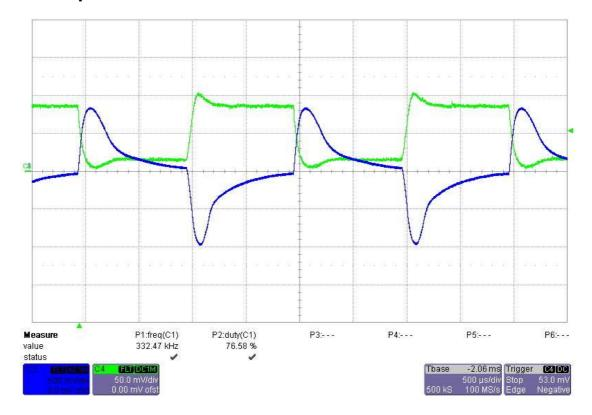
Fig.7 Output voltage (C3) AC variation, at step Load (C4)changing from 0.2A to 0.9A and viceversa @ Vin=48V.
