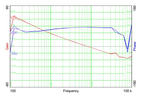
Fig.6 Open Loop Gain with full load and Vin = 36V and Vin=57V.
