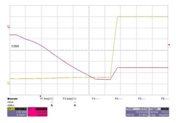
Fig.1 START-UP C1: Vout, C2: V\_aux\_power (scope probe on J1-, no GND)
