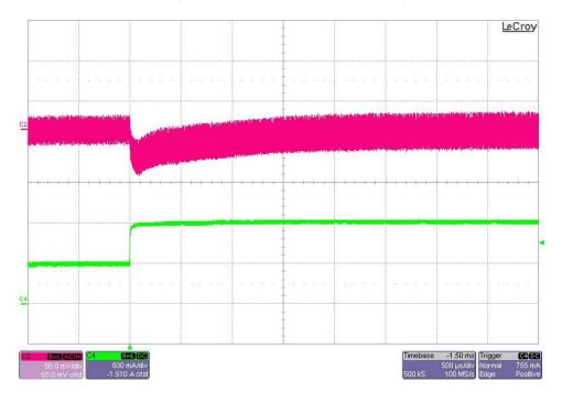
The photo below shows the 5V output voltage (top, ac coupled) when the load current is stepped between 1A and 0.5A. Vin = 4.0Vdc (50mV/DIV, 500mA/DIV, 500uS/DIV)
