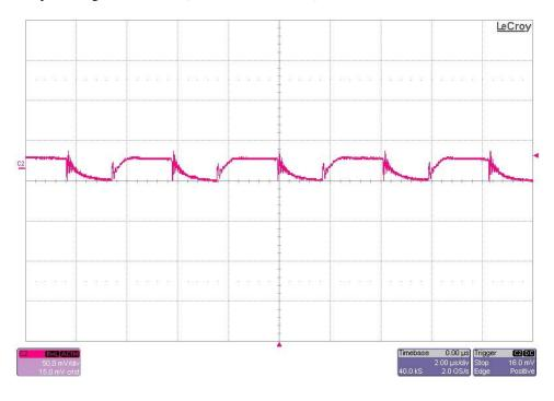
The 5V output ripple voltage is shown in the figure below. The image was taken with the output loaded to 1A and the input voltage set to 3.5Vdc. (50mV/DIV, 2uS/DIV)
