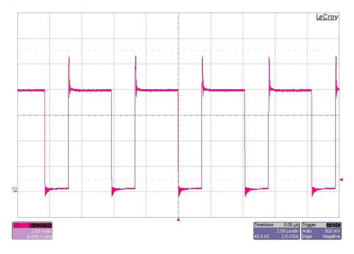
The photo below is the N-ch FET drain waveform. The input voltage is 5.25V and the output is loaded to 140mA. The converter has started discontinuous operation. (2V/DIV, 2uS/DIV)
