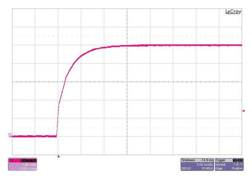
The photo below shows the 5V output voltage startup waveforms after the application of 4Vdc in. The output was loaded to 1A. (1V/DIV, 5mS/DIV)
