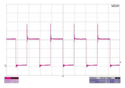
The photo below is the N-ch FET drain waveform. The input voltage is 3.5V and the output is loaded to 100mA. The converter has started discontinuous operation. (2V/DIV, 2uS/DIV)
