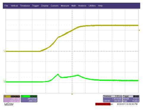
The scope plot below shows the 5V output voltage startup waveform after the application of 48Vdc at J1 (Ethernet connector. The output was loaded to 4.5A using an electronic load in CR mode.
