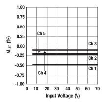
Current regulation (channel-to-channel) vs V<sub>IN</sub>.
