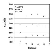
Current regulation (channel-to-channel) vs temperature.
