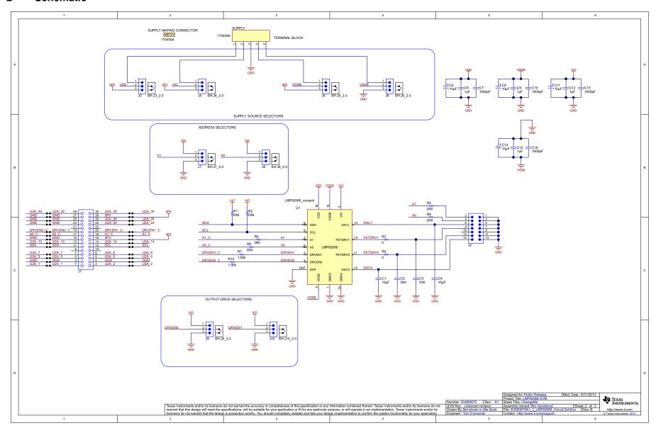
Figure 11. LMP92066EVM Schematic
