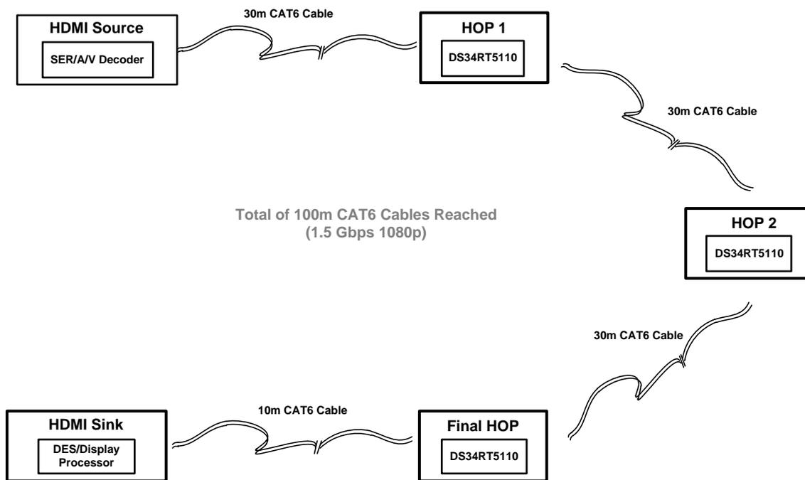
Figure 13. Multi-hop System (1.5 Gbps — 1080p, Total Cable Reach = 100m CAT6)
