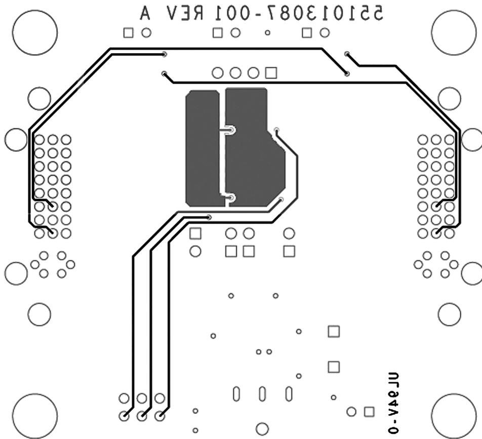
**Figure 19. DS16EV5110A Evaluation Board Layout (with DVI Connectors) – Bottom Side**
