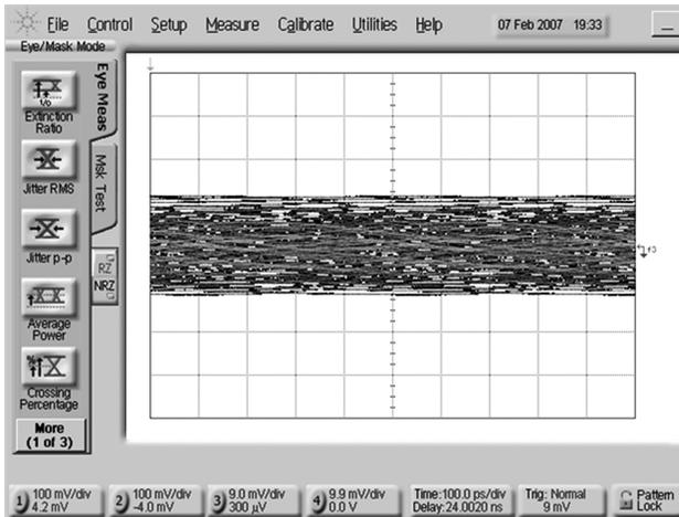
Figure 1. Eye Diagram After 25m 28 AWG DVI Cable (1.65 Gbps)
