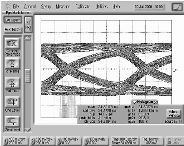
Figure 3. Eye Diagram After 5m 28 AWG DVI Cable (1.65Gbps)
