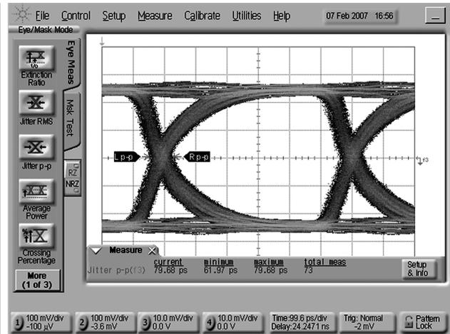
Figure 2. Output Eye Diagram of DS16EV5110A w/ 25m 28 AWG DVI Cable (1.65 Gbps)
