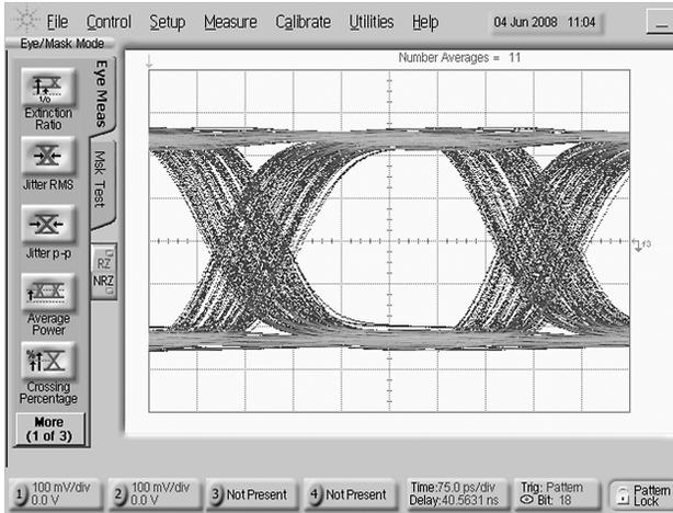
**Figure 9. Eye Diagram at TPC w/ EQ Only (2.25 Gbps, Cable A = 25m 28 AWG HDMI)**
