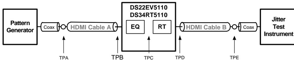
Figure 6. Simplified Test Setup as a Single Repeater
