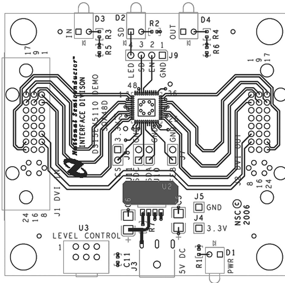
Figure 18. DS16EV5110A Evaluation Board Layout (with DVI Connectors) – top side
