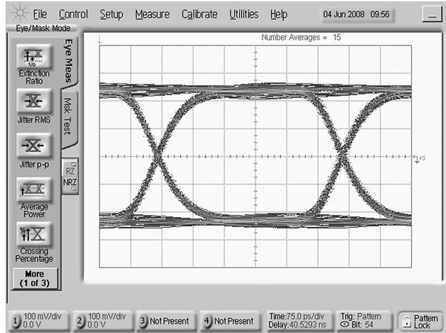
**Figure 10. Eye Diagram at TPD (2.25 Gbps, Cable A = 25m 28 AWG HDMI)**
