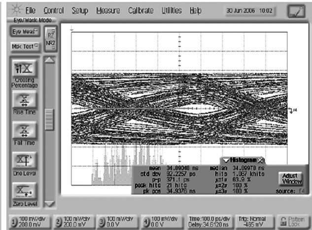
Figure 4. Eye Diagram After 10m 28 AWG DVI Cable (1.65Gbps)
