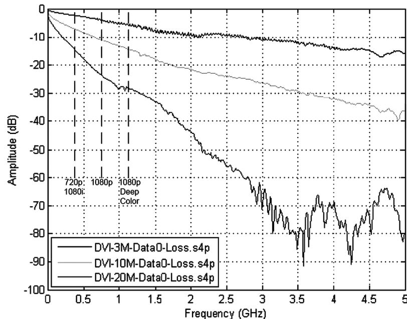
Figure 5. Transmission Loss of 3-, 10- and 20-Meter DVI Cables (28 AWG). Vertical lines drawn at 720p/1080i, 1080p60, and Deep Color 1080p60.
