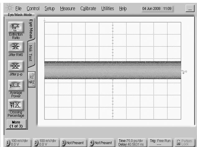
Figure 8. Eye Diagram at TPB (2.25 Gbps, Cable A = 25m 28 AWG HDMI)
