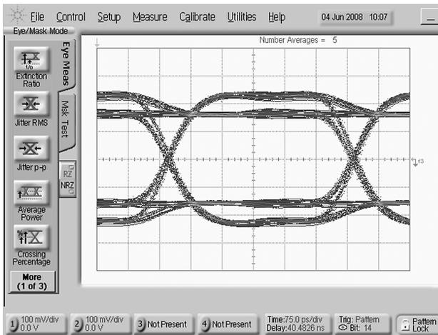
**Figure 11. Eye Diagram at TPD w/ DE on (2.25 Gbps, Cable A = 25m 28 AWG HDMI)**
