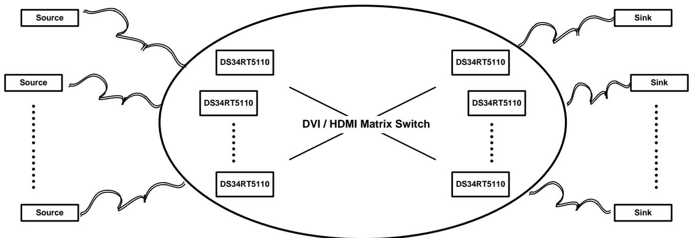
Figure 14. Complex HDMI Matrix Switch System
