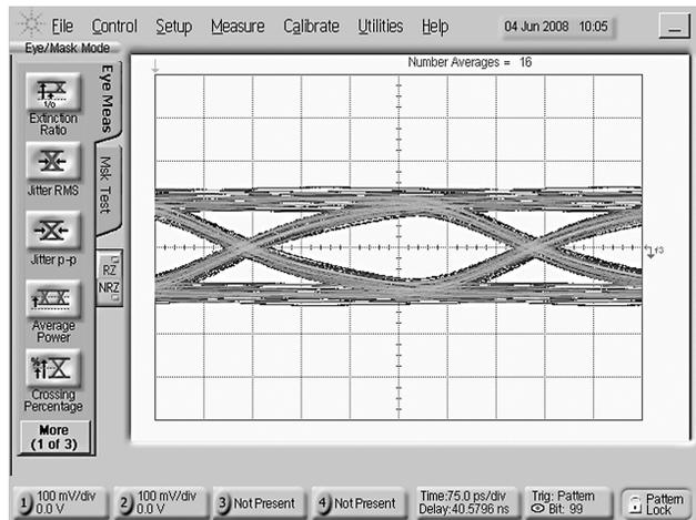
**Figure 12. Eye Diagram at TPE w/ DE on (2.25 Gbps, Cable A = 25m, and Cable B = 7.5m 28 AWG HDMI)**
