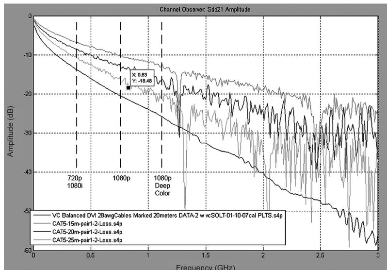
Figure 17. Transmission Loss of 20-Meter DVI Cable, 15-, 20- and 25-Meter CAT5 Cables
