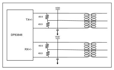
Figure 2. DP83848 PMD Connections (Termination)
