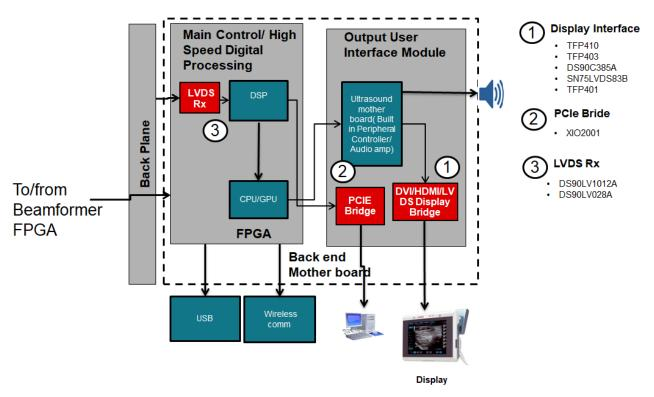
Figure 4. DSP and User Interface Subsystem
